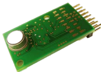
Figure 1. Sensor module for IAQ monitoring - micromachined MOS gas sensor.
