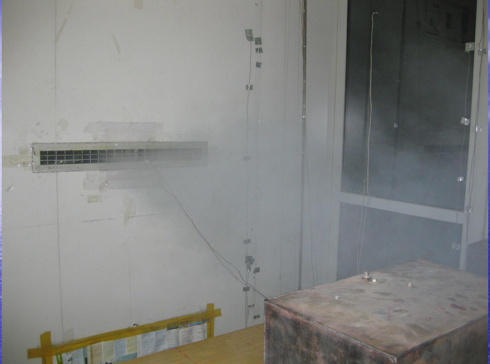
Air supply stratum formed under heating condition
