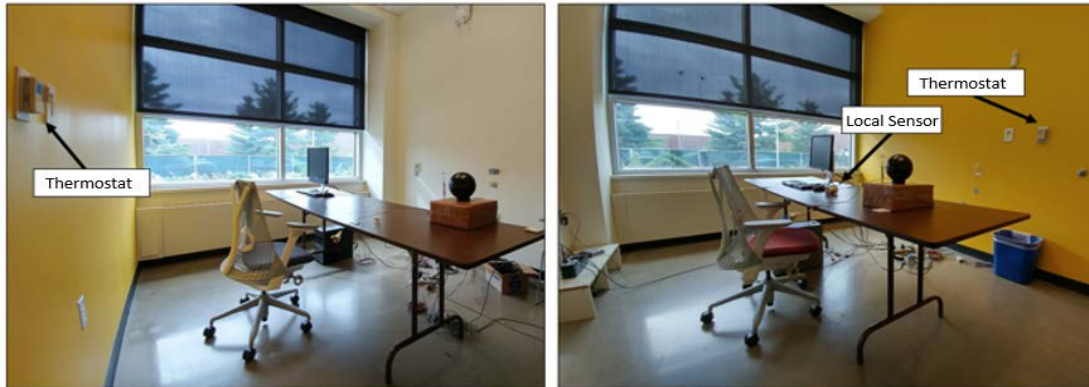
Figure 8 Experimental setup in two adjacent, identical private offices for comparing the performance of temperature control using a local sensor vs a wall thermostat.
