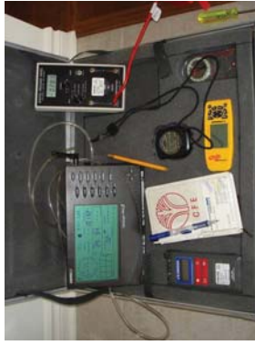
Figure 11: Monitoring panel equipped with remote weather station receiver and digital micro manometers.
