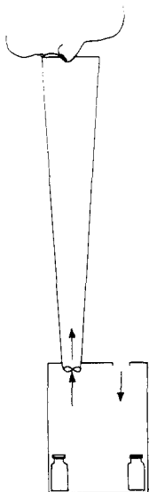
Figure 2 The decipolmeter. By varying the number of bottles with 2-propanone and the diameter of the hole in the top of these bottles different concentrations can be established.
