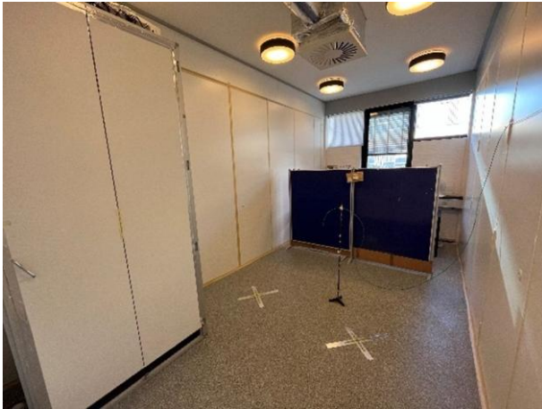
Figure 1: Test room with partition to hide pollution sources and air cleaners
