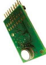
Figure 1. Sensor module for IAQ monitoring - micromachined MOS gas sensor.
