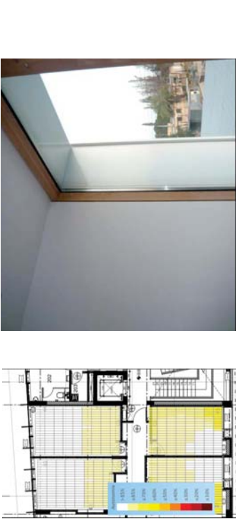
Figure 8. Natural light autonomy, simulated with DIAL+ software between 75 and 85% during working hours.
