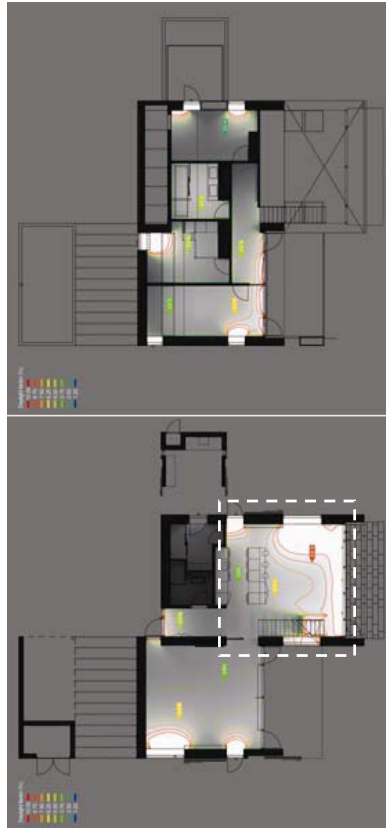
Figure 1. Calculated daylight factors in "Home for Life". Ground floor on the left, and upper floor on the right. The dotted rectangle indicates the kitchen and dining room which will be investigated in details.
