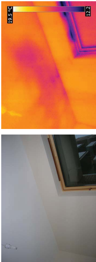
(a) Photograph taken of the junction between the wall and ceiling above a window in one of the bedrooms of the test flat (b) Thermal image shows localised surface temperature decrease in ceiling area corresponding with the position of the extract duct for the mechanical ventilation unit
