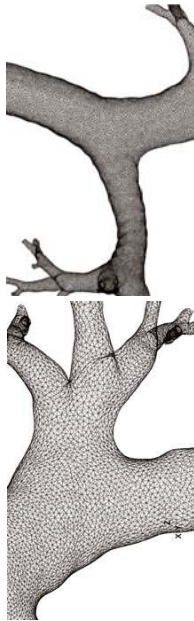
Figure 3 Detailed Grid Design of Airway Model
