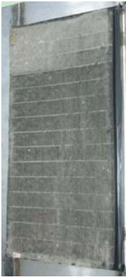
Figure 6a. F7 filter not protected (1 year), system A.
