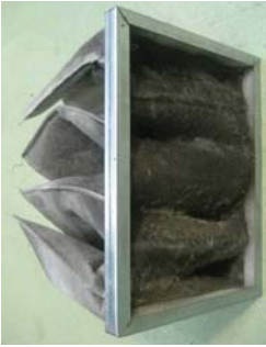
Figure 9b. G4 filter (1 year), system B.
