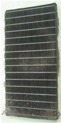
Figure 7a. F7 filter protected (1 year), system A.
