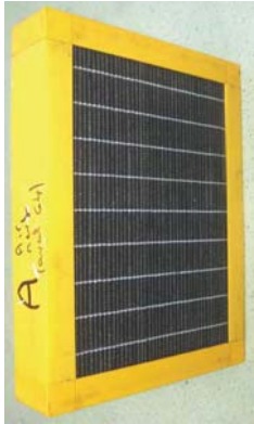
Figure 7b. F7 filter protected (1 year), system B.
