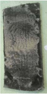
Figure 9a. G4 filter (1 year), system A.
