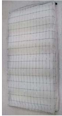
Figure 1a. System A : G4 filter.
