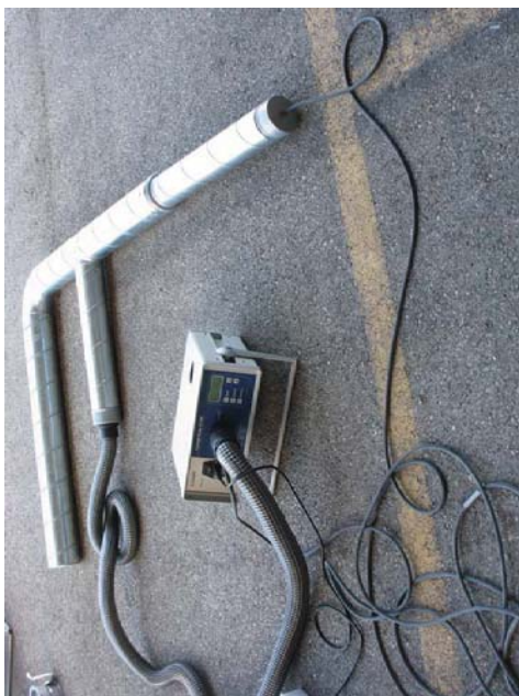
Figure 3 : Example of air tightness test
