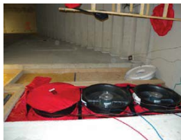
Figure 5. BlowerDoor MultipleFan (3 fans) in the stairwell
