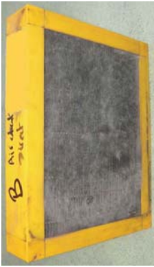
Figure 6b. F7 filter not protected (1 year), system B.
