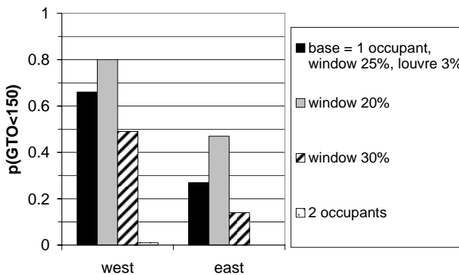
Fig. 5.39 Comparison of the impact of window area and occupancy on the probability of thermal comfort based on GTO
