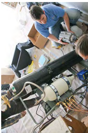
Figure 7: System developed by UC Davis, capable of multiple aerosol injection points
