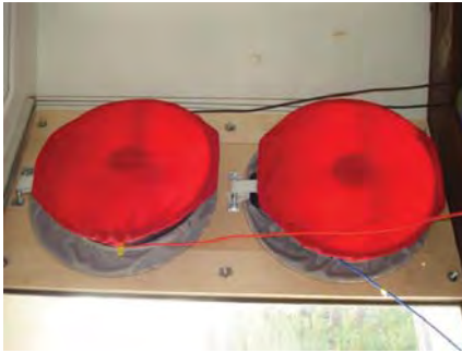
Photo 8: Custom-built blower door frame installed in a window opening.
