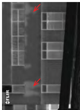
Figure 5: Convective heat loss pattern noted below windows (building under negative pressure).
