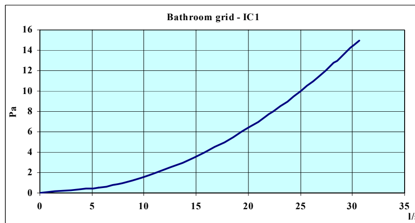
Figure 7-8 - Bathroom exhaust device characteristic
