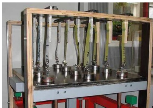
Figure 3: BRE Digest protocol for a mechanical ageing test (left) and the corresponding experimental set up of Ackermann (right)
