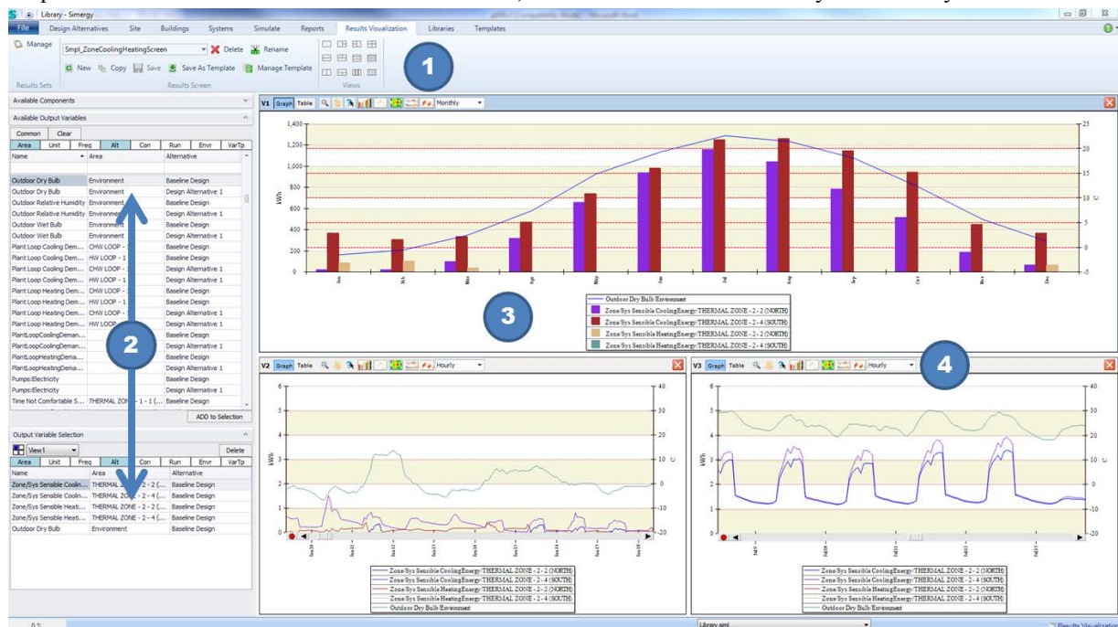
Figure 4: Layout of the visualization screen in the Simergy Interface including access to context specific data
