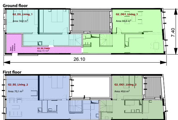
Figure 12 Ground plan of the regarded residential building.
