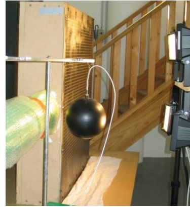
Fig. 2 Experimental set-up photograph: Radiation lamps and a perforated panel
